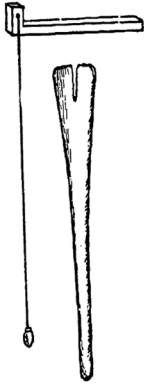
Figure 3. EGYPTIAN SIGHTING INSTRUMENT, THE MERKHET. After Borghardt.
