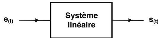
$$b_0 s(t) + b_1 \frac{ds(t)}{dt} + b_2 \frac{d^2 s(t)}{dt^2} + \dots + b_n \frac{d^n s(t)}{dt^n} = a_0 e(t) + a_1 \frac{de(t)}{dt} + a_2 \frac{d^2 e(t)}{dt^2} + \dots + a_m \frac{d^m e(t)}{dt^m}$$
